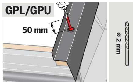
**ENGLISH:** Remove cover screws except the top cover screw **a**. The number of screws depends on the size and type of the window. Do **not** remove side frame covers **b**. If there is a mark at the top instead of a hole, drill hole through mark **c**. Place sealant on **all** screw holes **d**.
