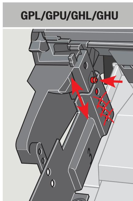
**ENGLISH:** Lower the roller shutter top casing as much as possible. Do **not** press the top casing against the roofing material **[a]**, **[b]**.
