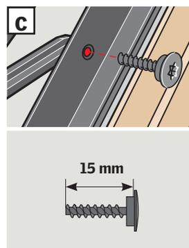
**ENGLISH:** Push side channels into position [a](#) and lay down on side covers [b](#). Attach opening restrictors to side covers with screws [c](#).
