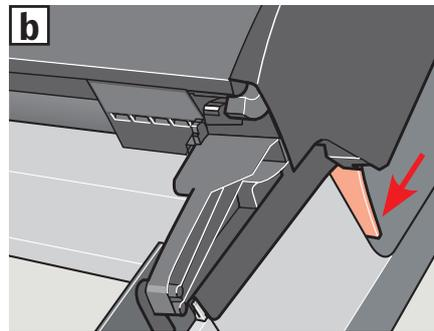
**ENGLISH:** Fit roller shutter top casing into grooves on side covers **[a]**. Check that rubber gasket at the back fits smoothly against outside of window **[b]**.
