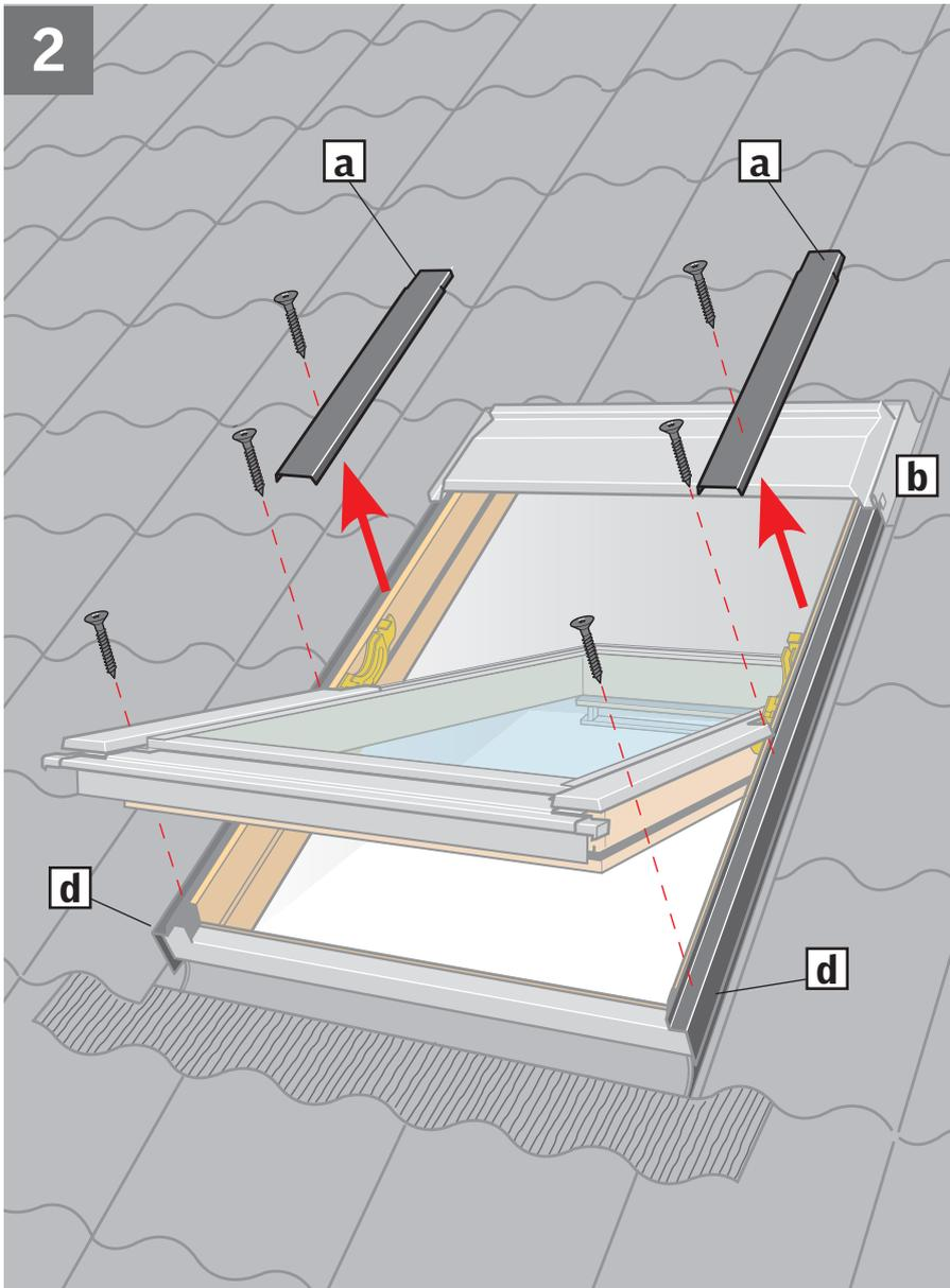
**ENGLISH:** Remove covers indicated temporarily **a**. Note the position of the covers for later refitting. Remove cover screws except the top cover screw **b**. If there is a mark at the top instead of a screw, drill hole through mark **c**. Do **not** remove side frame covers **d**. Place sealant on **all** screw holes **e**.
