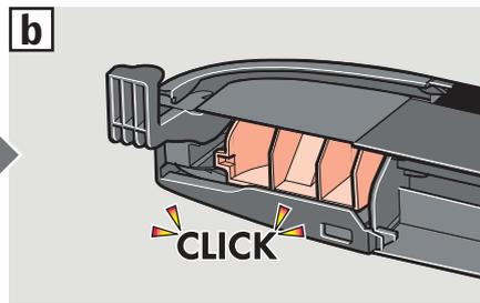
**ENGLISH:** Fit plastic insert pieces on the roller shutter side channels [a](#), [b](#).
