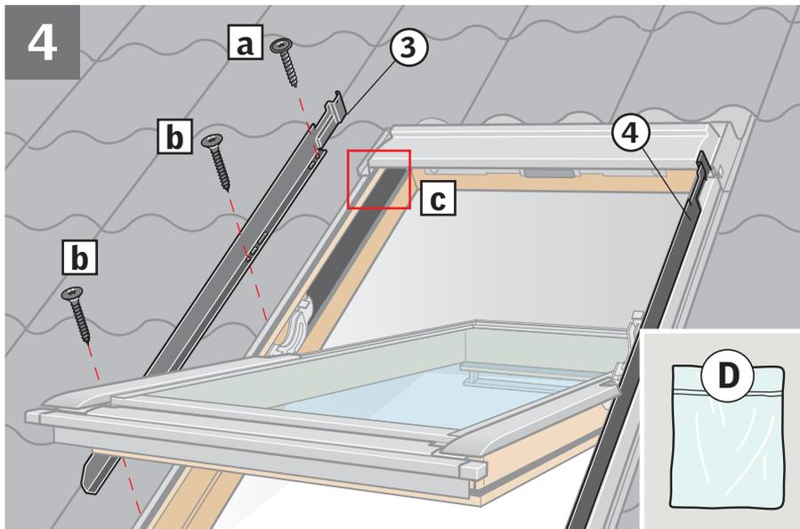
**ENGLISH:** Fix roller shutter side covers in the round holes with screws [a](#), [b](#).
