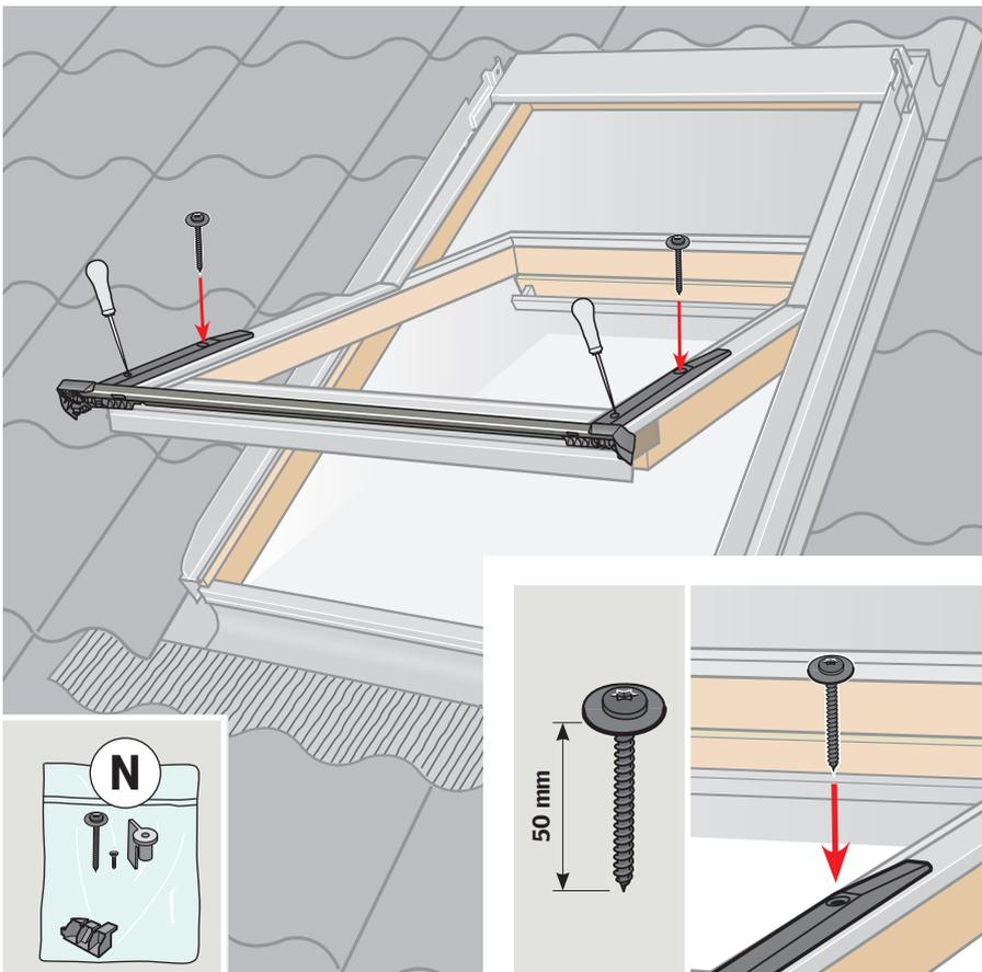
**ENGLISH:** Fit storm brackets and bottom cover temporarily with screws in the upper holes. Make a mark with bradawl through the lower holes.
