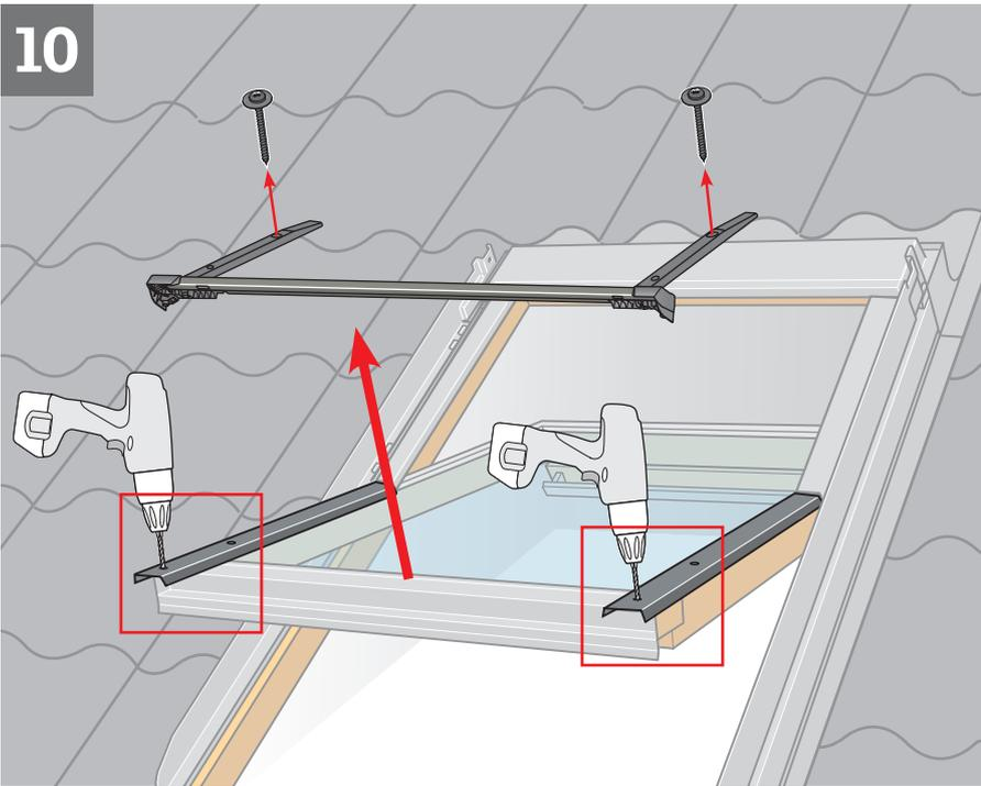
**ENGLISH:** Remove bottom cover temporarily and drill lower holes **[a]**. Place sealant on **all** screw holes **[b]**.
