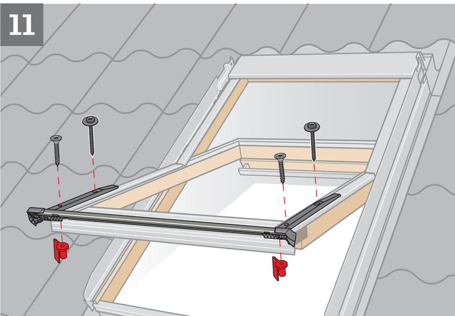
**ENGLISH:** Fit bottom cover. Secure lower screws with special nuts.
