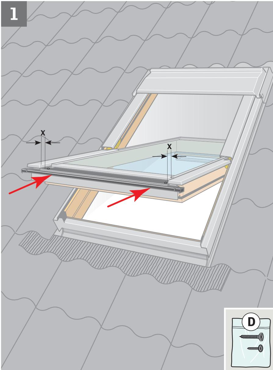
**ENGLISH:** Position bottom cover and push up against bottom edge of profile. Distance **X** must be the same at both sides. Make a mark with bradawl through holes in bottom cover **a**. Drill  $\varnothing 2$  mm holes **b**. Fit bottom cover **c**.
