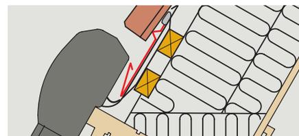
**ENGLISH:** If the roller shutter is to be installed with flashing EDJ or EDN: Bend down rainwater deflector to make room for roller shutter.
