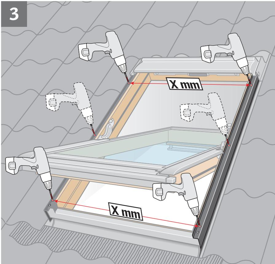
**ENGLISH:** Drill a hole through the marks in the side frame covers [a](#). To ensure that the roller shutter runs efficiently, the distance (**X mm**) between the side frame covers at top and bottom must be exactly the same.
